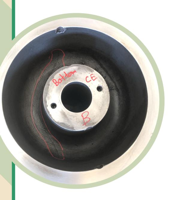
During a routine overhaul, an olefins manufacturer in Thailand noticed some problems on their Belliss & Morcom Recycle Hydrogen Compressor. Both the pistons of the single stage compressor were cracked on the head end, indicating mistakes made during the last overhaul of the compressor.
