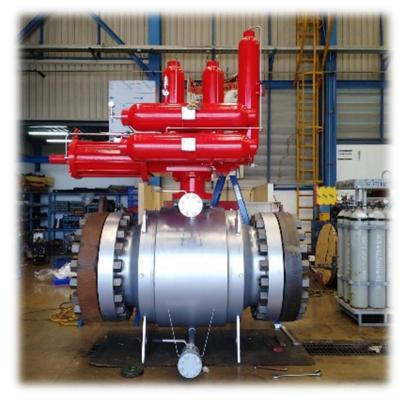
PSS successfully delivered and commissioned 30" Trunnion Mounted Welded Body API 6D Class 900 ball valves to a major PTT company. This valve was installed on a hot tapped pipeline which would de-bottleneck the main pipeline where an existing Perar Ball Valve is already installed.
