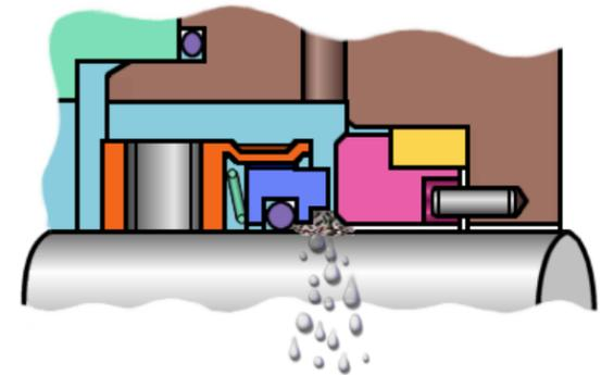
John Crane 680 is "Non Pusher Seal" The tail end of the bellows is held tight to the shaft forming a static (O-ring) seal. The other end of the bellows "floats" above the shaft and pushes against the primary ring. The flexibility of the bellows type 680 allows for seal face wear and for shaft misalignment better than Flowserve RO seal and eliminated seal hang up problem for Sodium Hydroxide application. However, for this application required install seal plan 62 with clean water quenching too.
