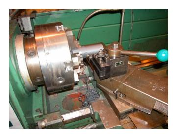
Vespel® CR-6100 comes off the tool like a ribbon of tape during machining
